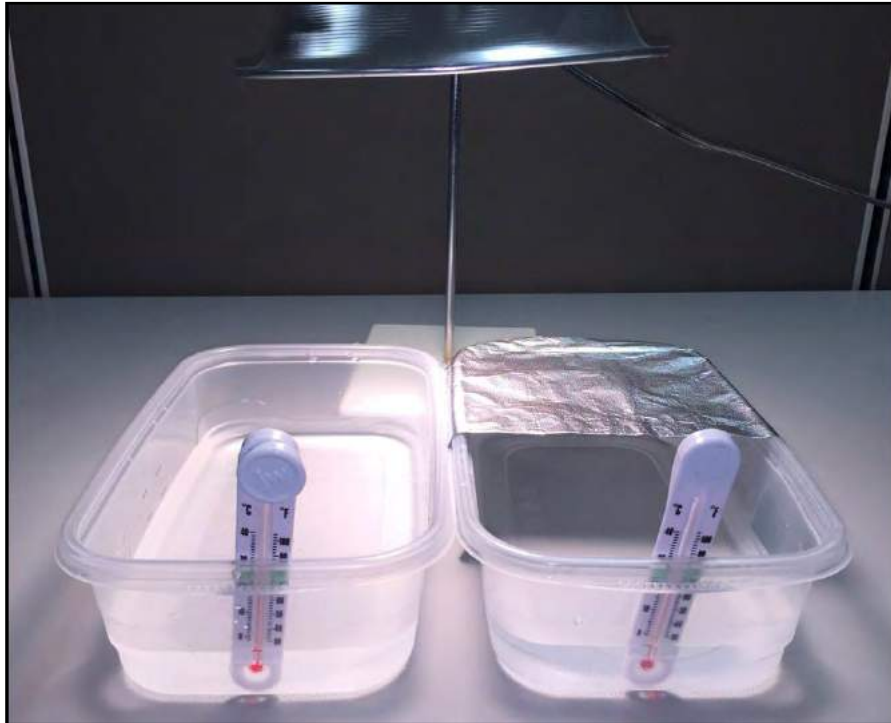
Figure 13. Example of an experimental setup for determining the relationship between water temperature and sea ice.
