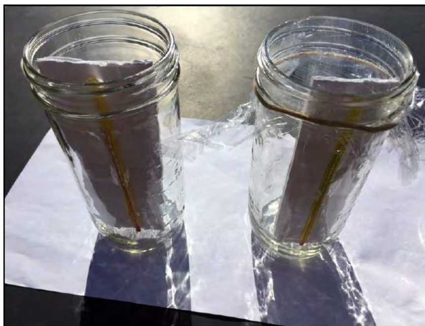
Figure 11. Model #1 with no covering and Model #2 covered with clear plastic wrap secured by a rubber band.
