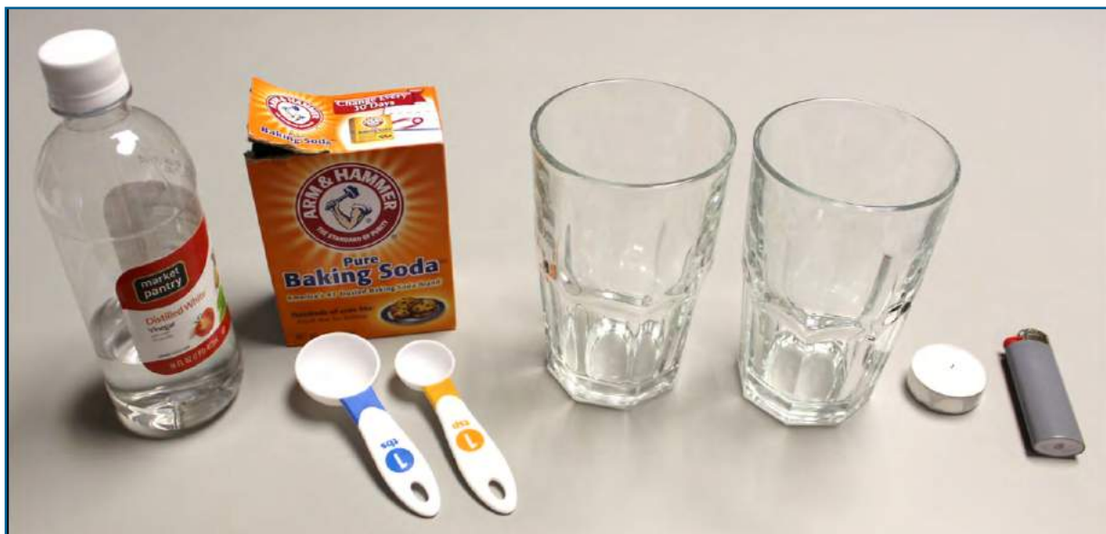
Figure 7. Materials for investigating the relative weight of carbon dioxide gas.
